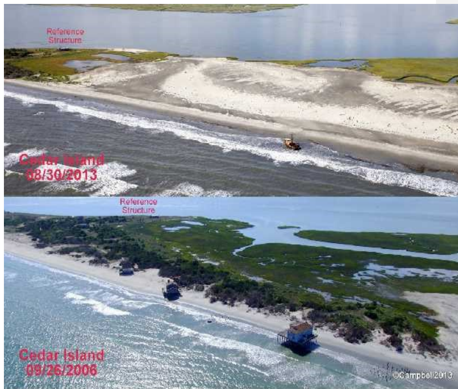
Photo Courtesy of Gordon Campbell, At Altitude Gallery Cedar Island has lost approximately \frac{3}{4} of a mile of its southern tip which has opened the Wachapreague Inlet very wide exposing the opposite bank of salt marsh to direct impingement by the ocean swells and waves which will eventually result in erosion and loss of the salt marsh habitat.
